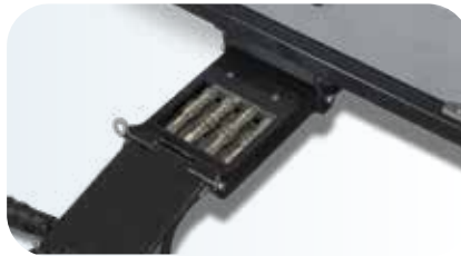
Quick couplings to configure the machine according to the job
